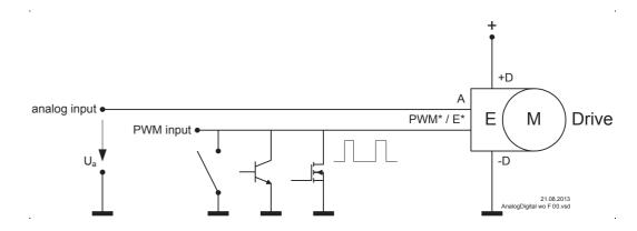
In this operating mode the supply voltage plus is usually connected permanently. To run the Drive on the pin PWM\* / E\* a PWM signal has to be applied and with the duty cycle of the PWM signal the Drive speed can be then controlled. If the pin PWM\* / E\* is switched to supply voltage minus the Drive speed can be then controlled with an analog voltage on the pin A. So a mixed control with either digital or analog input is possible. The priority has the digital PWM signal.
