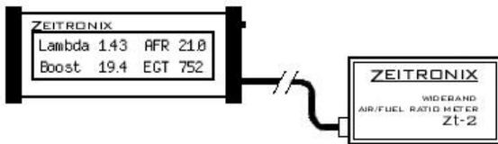
Connecting the Zt-2, PC and the AFRM Display through the provided serial data splitter
