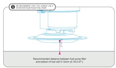
Mount the pickup pipe assembly to the CFC Unit top lid, make sure the fuel pump and fuel hose do not interfere with any of the functions of the top lid, and then tighten the hose clamp fully to fixate the fuel pump.
